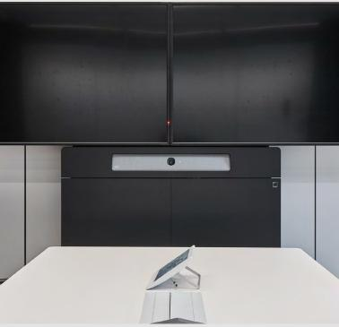
Mounting the Cisco Room Kits above the display works perfectly for all sizes of the Elements furniture W6, W8 and S1.
