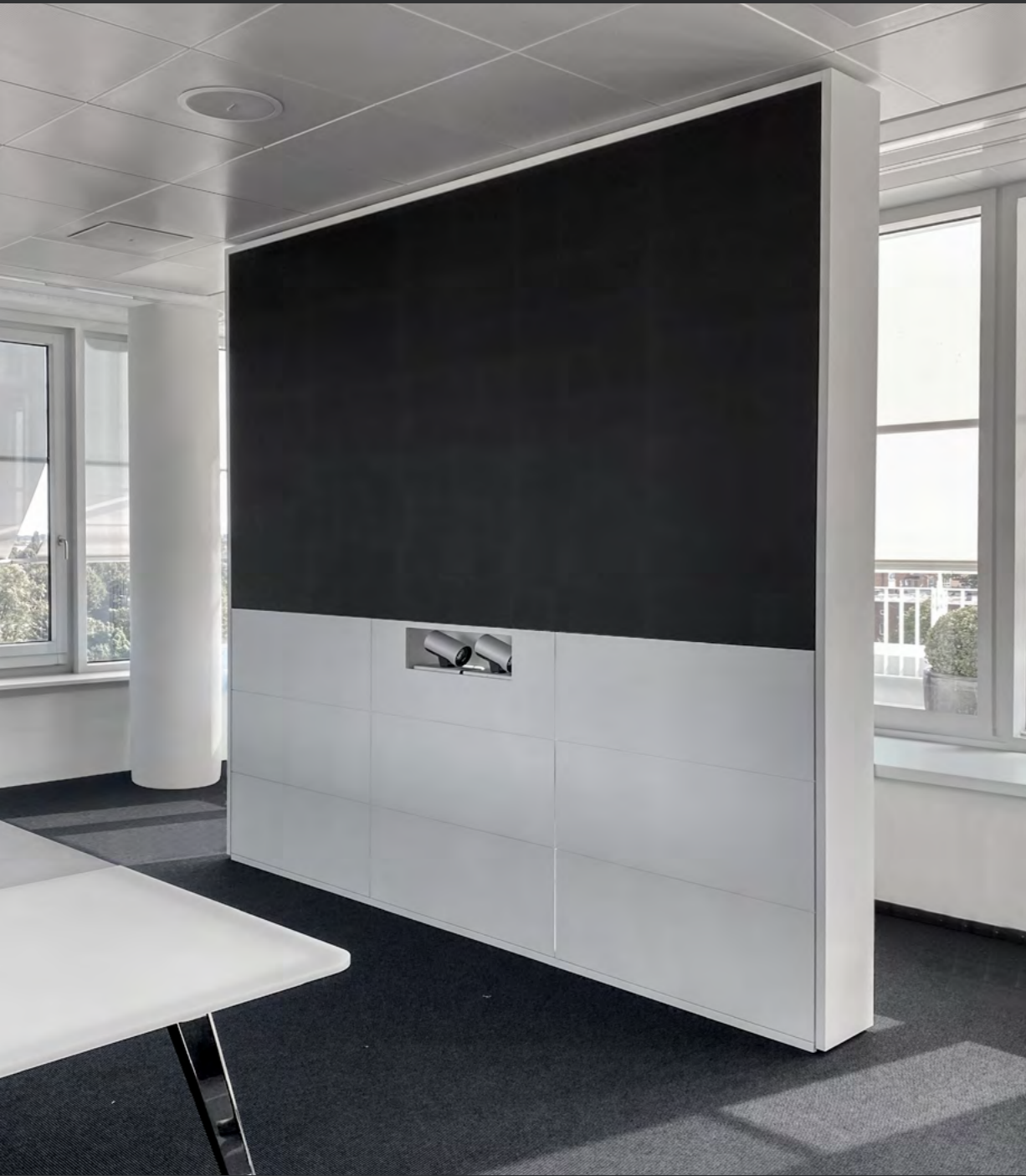
A freestanding 136" LED Media Wall in arctic white, custom-made for a board meeting room, with an integrated Cisco VC system (as well as loudspeakers in the ceiling).
