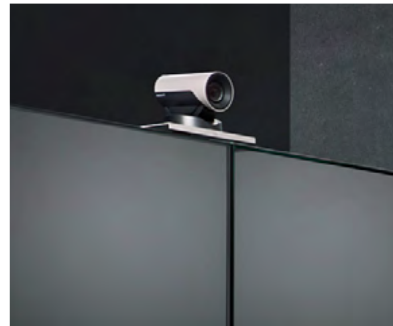
Mount for VC camera above the display
